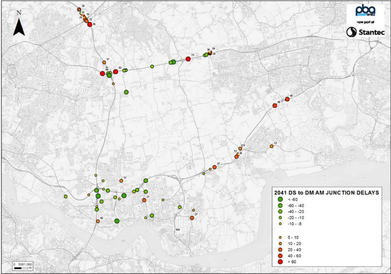
Figure 6.1: Differences in Delays in AM Peak Hour with LTC (Statutory Consultation Fixed Matrix Cordon Model)
